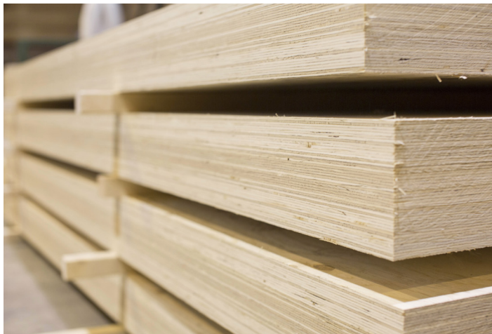
Figure 3.4. Storage of LVL packages
