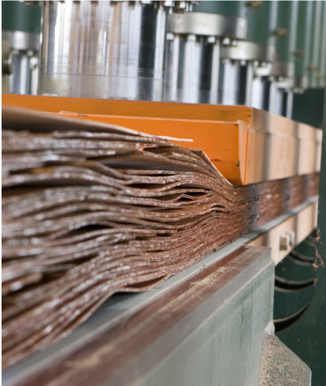
Figure 1.41. Pre-pressing: the billet is cold pressed to spread the glue evenly between the veneers.
