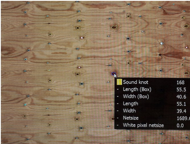
Figure 1.30. VDA camera image for visual defect analysis.
