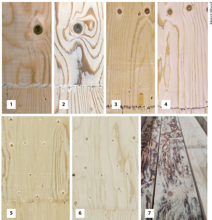
Figure 1.65: Appearance of LVL veneer surfaces 1. Unsanded front side, close image 2. Optical sanded front side, close image 3. Unsanded reverse side with dark scarf-joint glue line, close image 4. Optical sanded reverse side with dark scarf-joint glue line, close image 5. Unsanded front side, general view 6. Optical sanded front side, general view 7. Calibration sanding revealing the dark glue line 11 .
